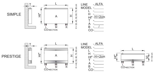
RADIATOR CONNECTION: if the connection of the radiator is on the RIGHT (R) side then the thermostatic head is on the RIGHT side of the radiator.
